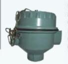
Material: Cast Aluminum Alloy LM6. Flameproof: Zone 1 & 2, GAS GROUP: IIA,IIB Finish: Light Grey to Shade 631 Gasket: Neoprene Cable Entry: 1 Nos. 3/4" ET Entry
